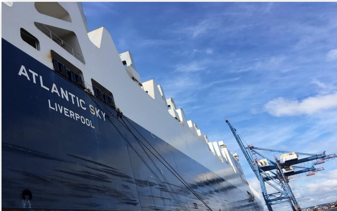
Picture 1: The Atlantic Sky is multipurpose roll-on/roll-off containership, designed to carry wheeled cargo, such as cars and trucks.
